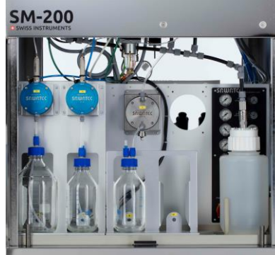
Additional dispensing line with dosing pump GSP-98
